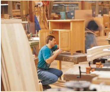
Pompanoosuc Mills craftsman Horace Pike installs the doors of a custom cabinet in solid cherry for a customer in New York City.
